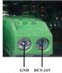
Figure 3-11 Wiring of Remote Input
