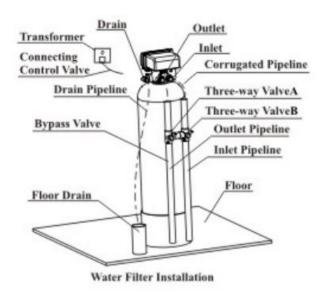
Illustration: Install two three-way ball valves to connect the control valve and inlet/outlet pipeline. The valve B is connected with the inlet of the control valve; the valve A is connected with the outlet of the control valve. When repair the tank, adjust the valve A and B to make the inlet connected with outlet directly, so the water do not pass through the valve; When normally use, adjust the vale A and B connected with valve.
